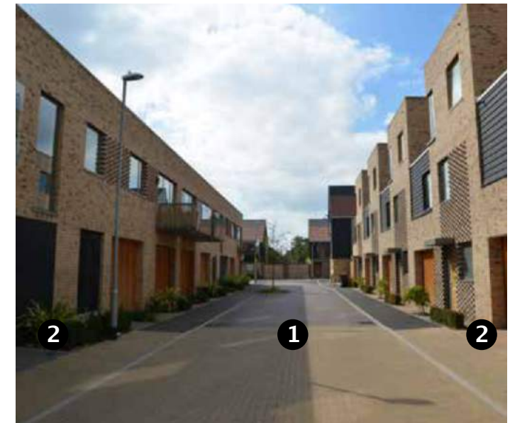
Figure 40: Example of a lane/private drive in Cambridge, with a shared surface for all road users.
